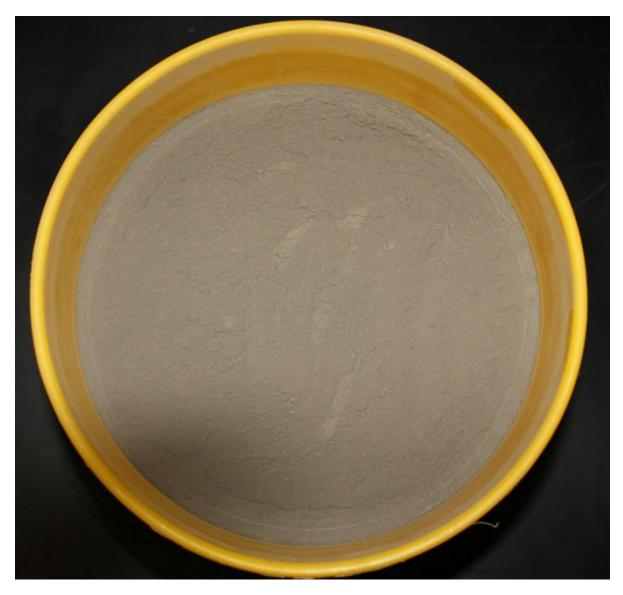
Photo 11 – Final bulk Puget Sound SRM (< 60 Mesh US Sieve) after rotary blending
